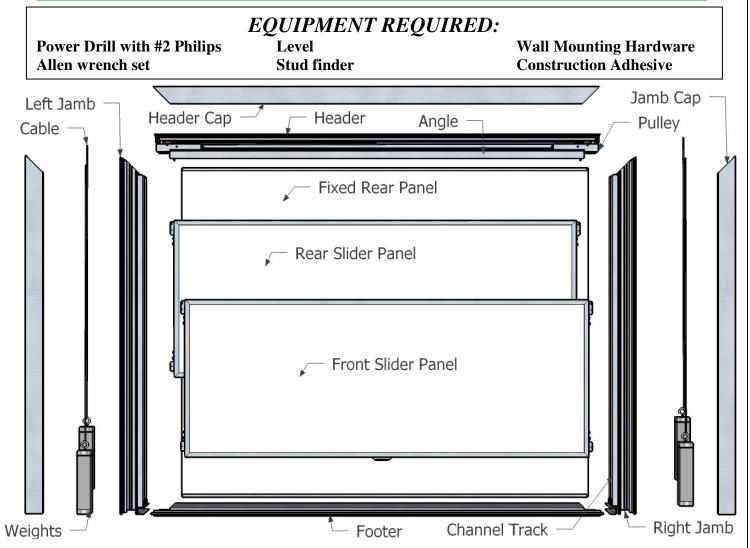
NOTE: Blocking is required at both housing **Jamb** verticals on center of the housing. Blocking for the **Header** is not required, but it must be installed into stud or block. (Large housing =  $2 \frac{1}{4}$ " in from overall width. Small Housing =  $1 \frac{3}{8}$ " in from unit width)
